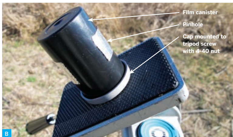
Fig. A: Pinhole sunshine recorder made from a plastic 35mm film canister. The blueprint paper is held in place by a thin strip of masking tape.
