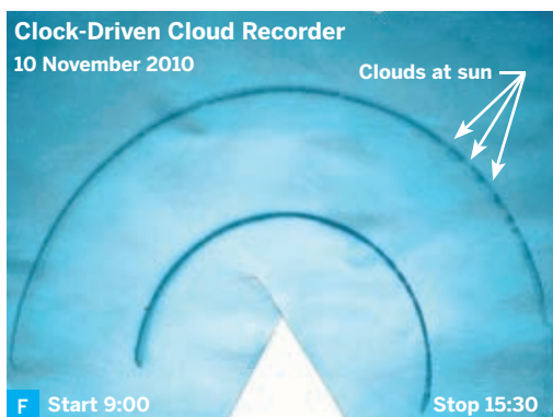
Fig. E: Quartz analog clock-driven recorder with two 1mm sunlight apertures. The black paper disk was taped to the clock's hour hand. Blueprint paper was taped to the clock face behind the black paper disk.
