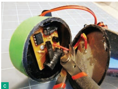
✂ Fig. E: Remove the screw to release the circuit board.
